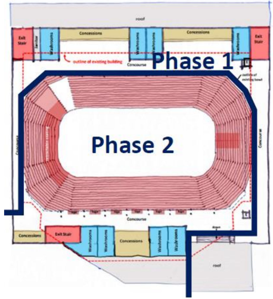
Figure 20 – Schematic sketch depicting the phasing of construction under a 2-phase construction schedule (Concourse Level)
