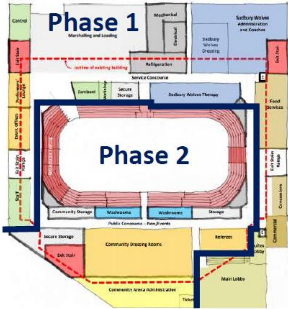
Figure 19 – Schematic sketch depicting the phasing of construction under a 2-phase construction schedule (Event / Entry Level)
