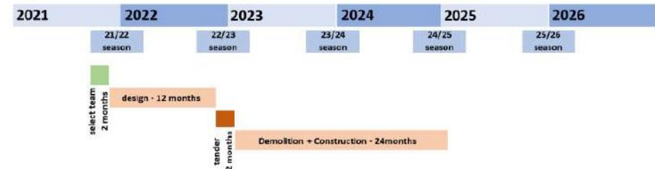
Figure 17 – Schematic schedule depicting the timeframes associated with modernizing the Sudbury Community Arena in a single phase
