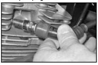
2. Turn engine switch to "ON". Start the engine. If the ignition system is operating properly, a blue spark should jump across the spark plug gap. If there is no spark, take your machine to your service center.
