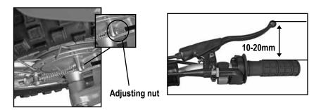
The front brake lever has a free operating movement of 10-20mm as shown.
